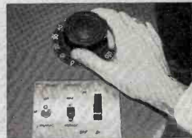
Individual switch and variable transformer control of each lamp allows quick switching or fading from transparencies to opaques.
